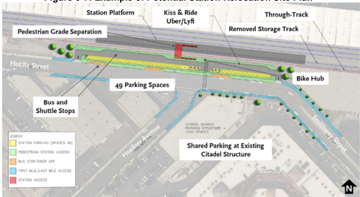
Figure 0-7: Example of Potential Station Relocation Site Plan
