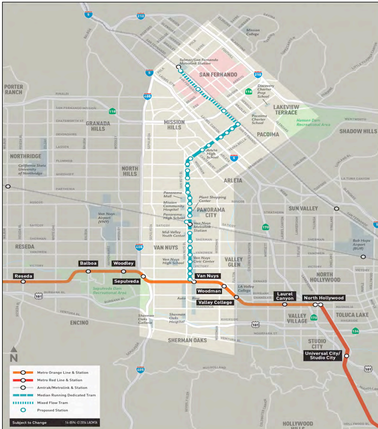
Figure ES-6: Alternative 3 – Low-Floor LRT/Tram
