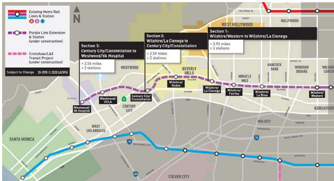
Figure 1: Purple Line Extension
