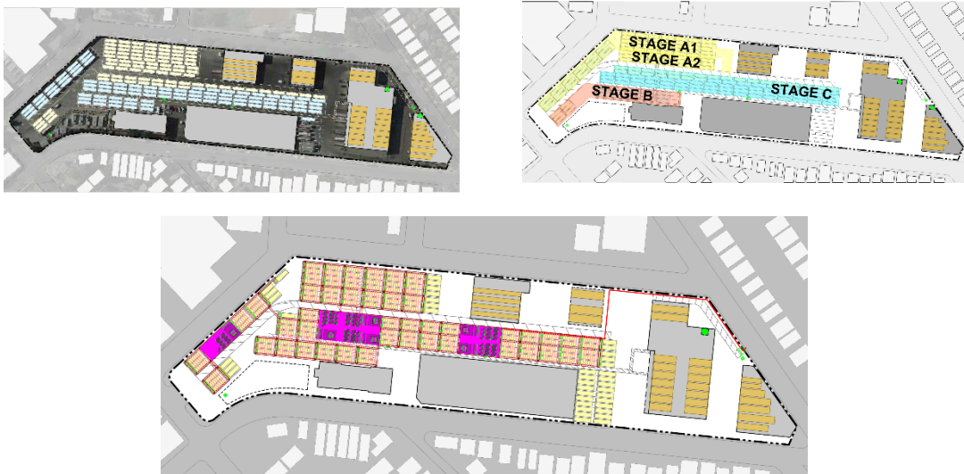
Figure 3-13. Division 3 – Existing, Construction Staging, and Buildout
