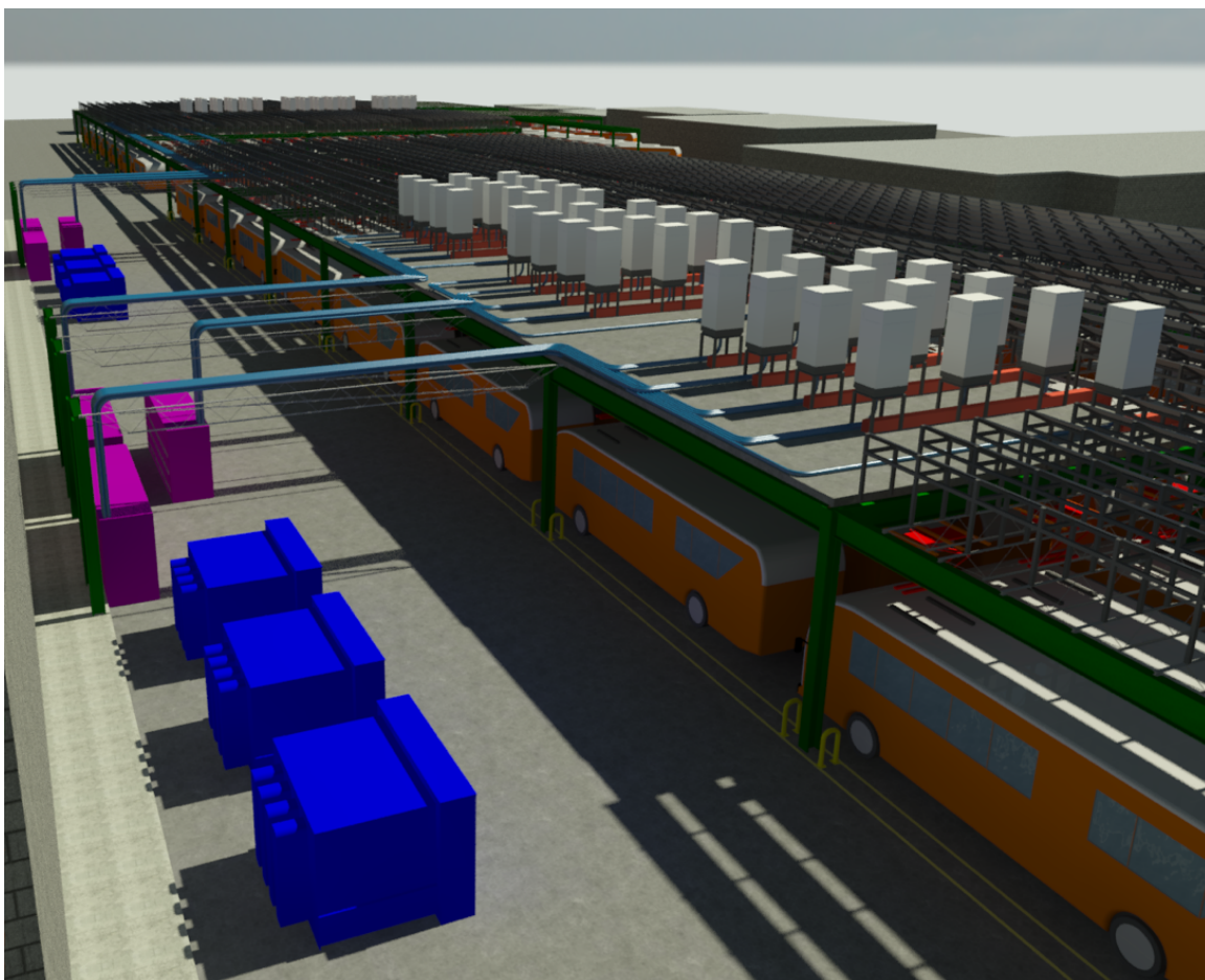
Figure 3-2. General Layout of Division Charging Infrastructure
