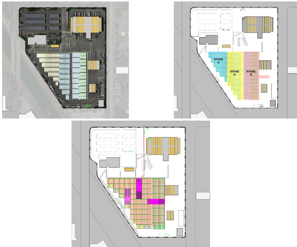
Figure 3-21. Division 18 – Existing, Construction Staging, and Buildout
