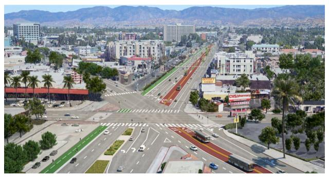
Figure 1: Center-running BRT on Vineland Avenue and Lankershim Boulevard in North Hollywood
