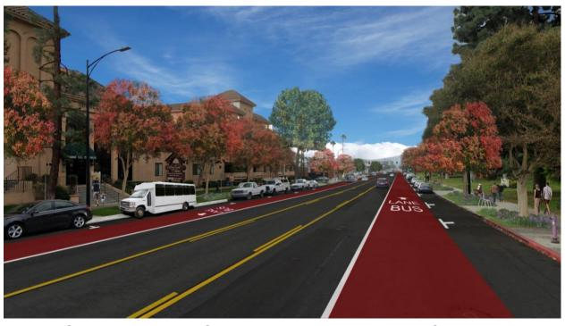
Figure 2: Side-running BRT on Olive Avenue between Buena Vista Street and Lake Street in Burbank
