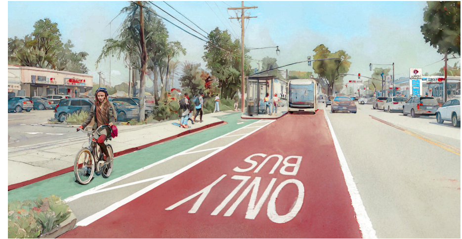
A rendering facing east, showing Side Running Bus Lanes on Garvey Avenue west of Santa Anita in El Monte
