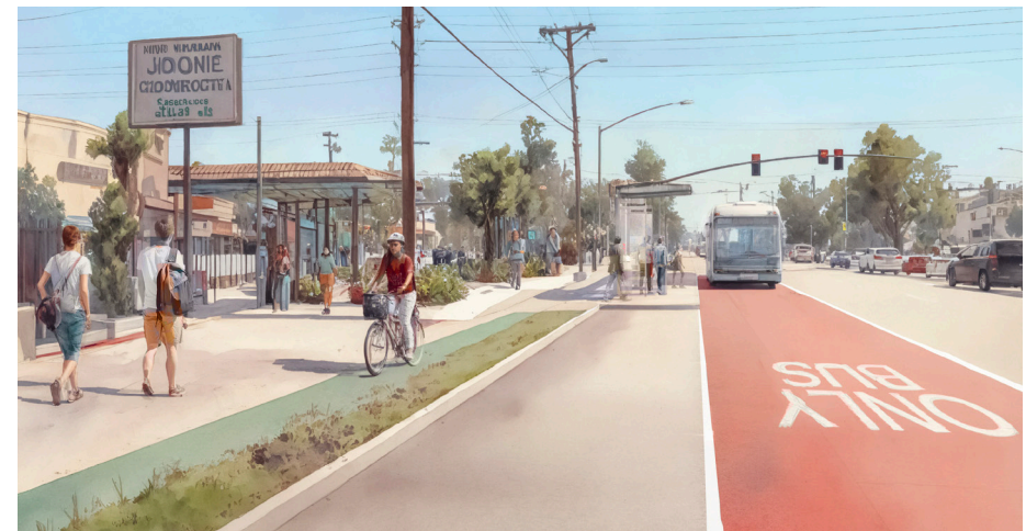
A rendering facing south, showing Side Running Bus Lanes with Protected Bike Lanes on Rosemead Boulevard at Rush Street in South El Monte
