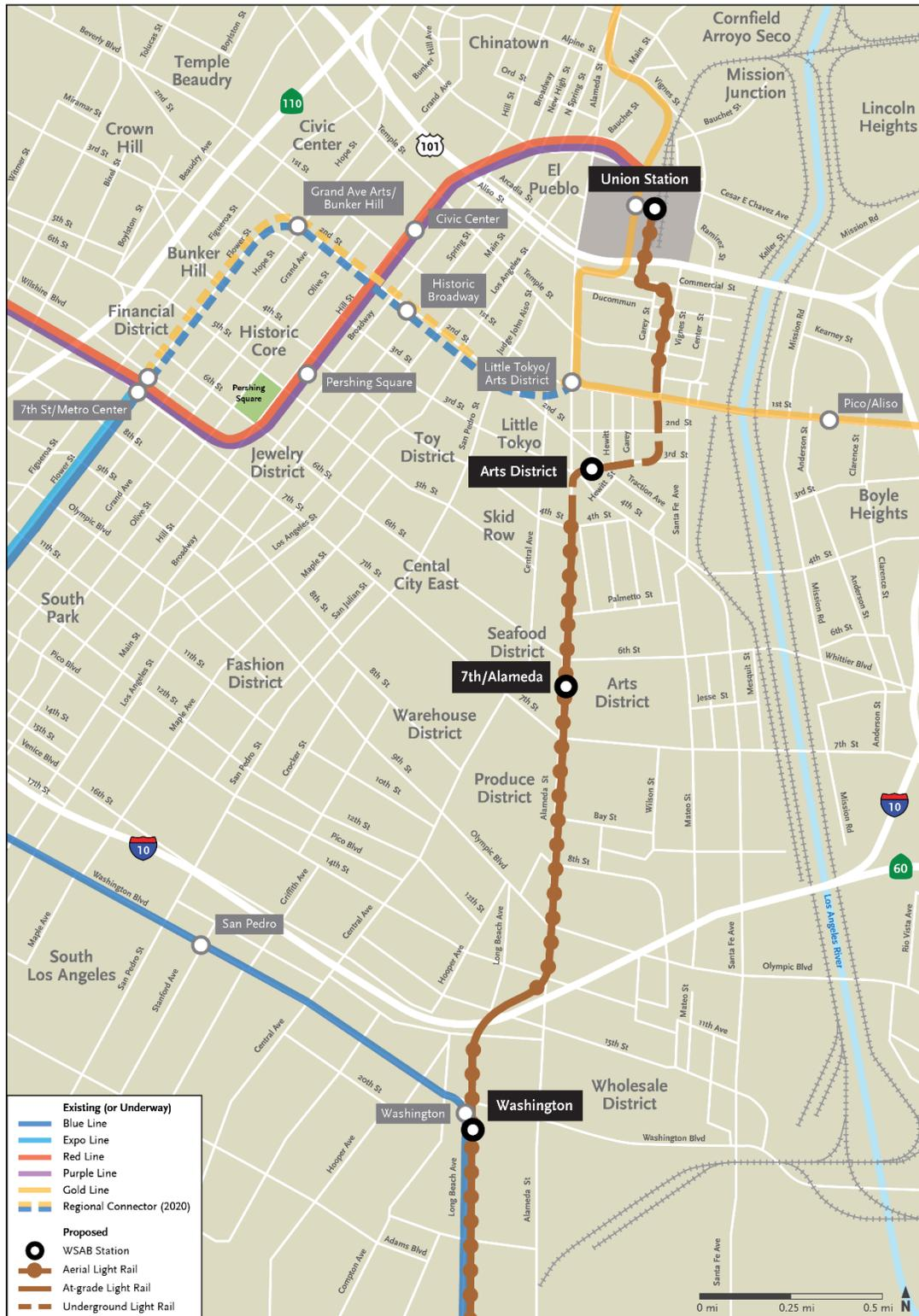
Figure ES-11. E) Alameda (underground) Northern Alignment Concept
