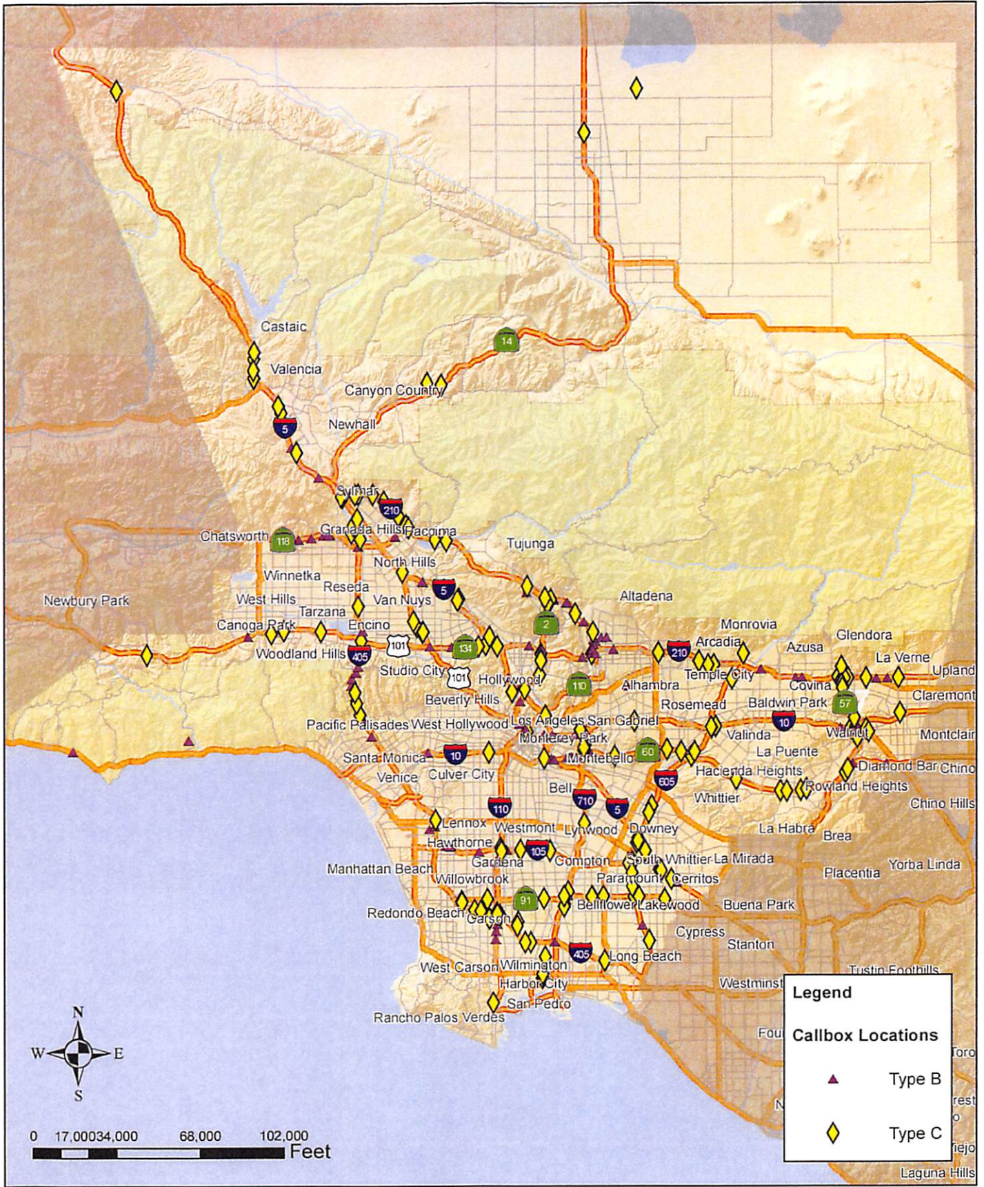
Los Angeles County SAFE Call Box Assessment Study
