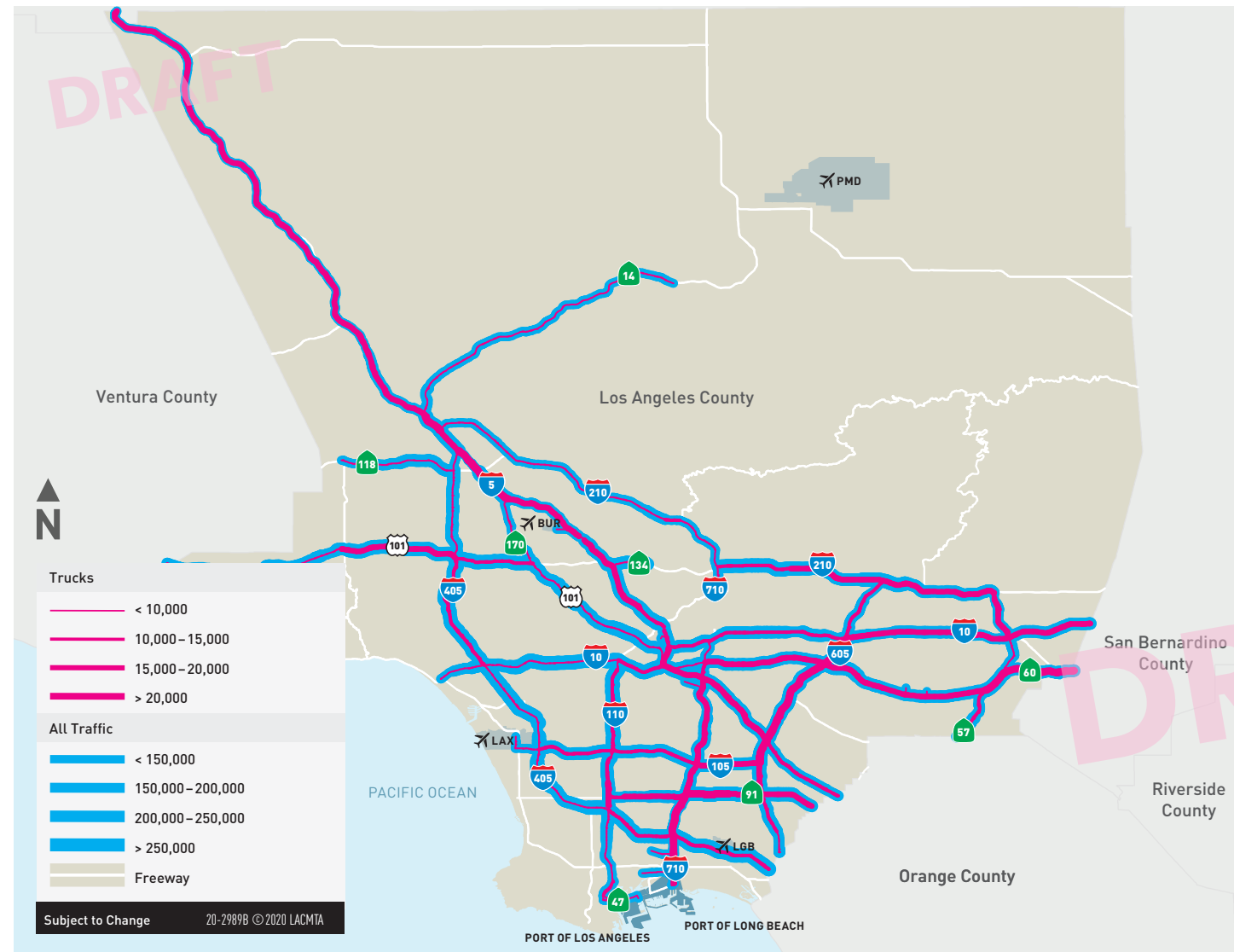
Figure 6 VOLUMES ON THE NATIONAL HIGHWAY FREIGHT NETWORK
