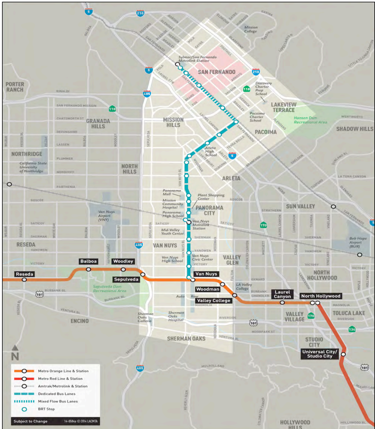
Figure ES-4: Alternative 1 – Curb-running BRT
