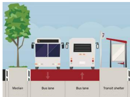
Median layout at staggered BRT station
